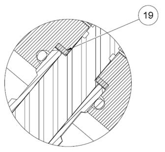
Washer Item 19 used on Plastic Diaphragm Plates Only Remove Washer Item 19 when installing Stainless Steel Diaphragm Plates
