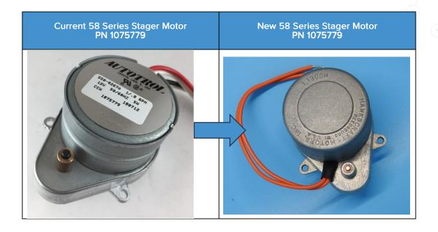
If manual rotation of the stager is required with the new motors shown above, the two motor mounting screws will need to be removed and the motor disengaged from the stager cam.
