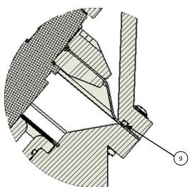
The Oring PN 1071713 will remain in Diaphragm and Seal Kits for the foreseeable future but will not be required if repairing valves with machined flat Cap and Body. The update will be implemented when inventory of the current version is exhausted.
