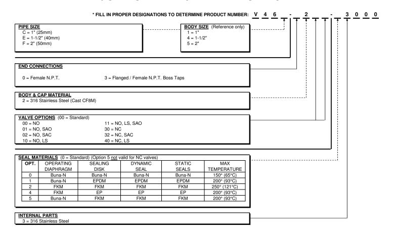
\* To create a valve number replace each "\_" with the proper number or letter for the feature you desire. For example, a 1" NPT Stainless Steel Valve Model V461 with Normally Closed and Spring Assist Closed Options is designated as a V46C-0232-03000.
